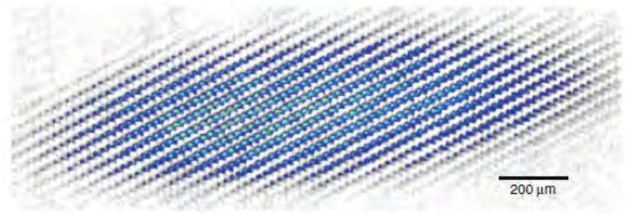
Absorption image of the loaded lattice, showing \sim 500 traps loaded with 200–2500 atoms each
